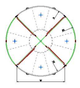
\*D : Outer diameter \*D2: Floor inner diameter \*W: Passage (mm) \*D1: Floor outer diameter
