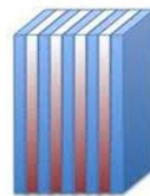
Bullet proof glass consisting of normal glass (blue) and polycarbonate (red) layers
